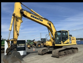
Komatsu PC240LC-11 Hydraulic Excavator
