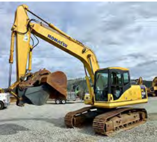
2005 KOMATSU PC160LC-7 excavator. Pre-emission Cummins 4BTA 3.9, new 36" dig bucket, link thumb, 60" cleanup bucket, wedge coupler, 80% undercarriage, AC, 7100 hours, excellent condition, $65,000. More pictures at www.GreatNorthernEquip.com or call 509-535-4427, Spokane
