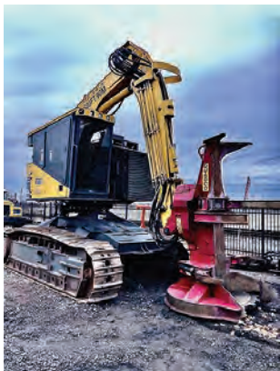
2017 KOMATSU XT445L-3 feller buncher. Quadco 24B 360 hot saw, 300HP Cummins, 6400 hours. Excellent condition, $265,000. More pictures at www.GreatNorthernEquip.com . Calls only, 509-535-4427, Spokane
